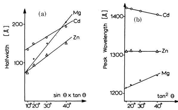
FIG. 2. Extrapolation of the photoemission values for Cd, Mg, and Zn to zero angle of incidence. (a) Plot of half width; (b) plot of peak frequency (dispersion).
