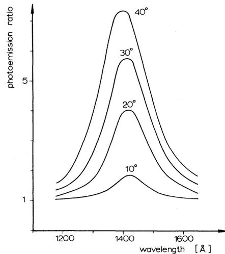
FIG. 1. Photoemission ratio of a 44-Å Cd film for several angles of incidence. Each curve has been normalized with the normal-incidence curve.
