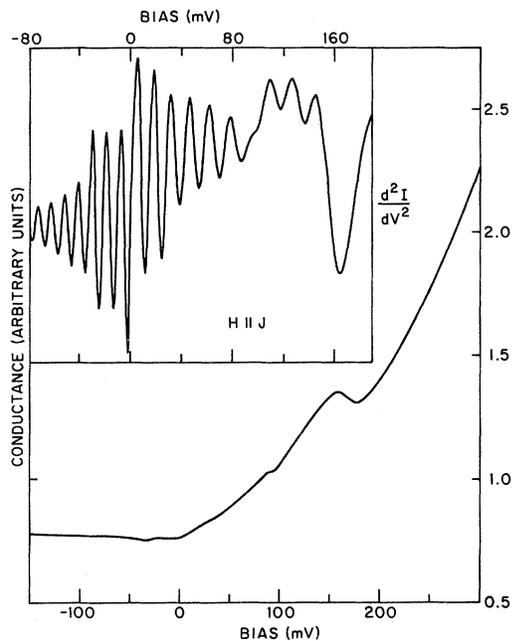
FIG. 1. The conductance-versus-bias curve of an  $n$ -type InAs-oxide-Pb (normal state) tunnel junction at 4.2°K. The InAs is degenerate, having bulk electron concentration  $n \approx 5.5 \times 10^{17}/\text{cm}^3$ . The bias sign refers to that of the Pb electrode. The insert shows the  $d^2I/dV^2$  versus bias curve when a magnetic field (35 kG) is applied normal to the junction surface.
