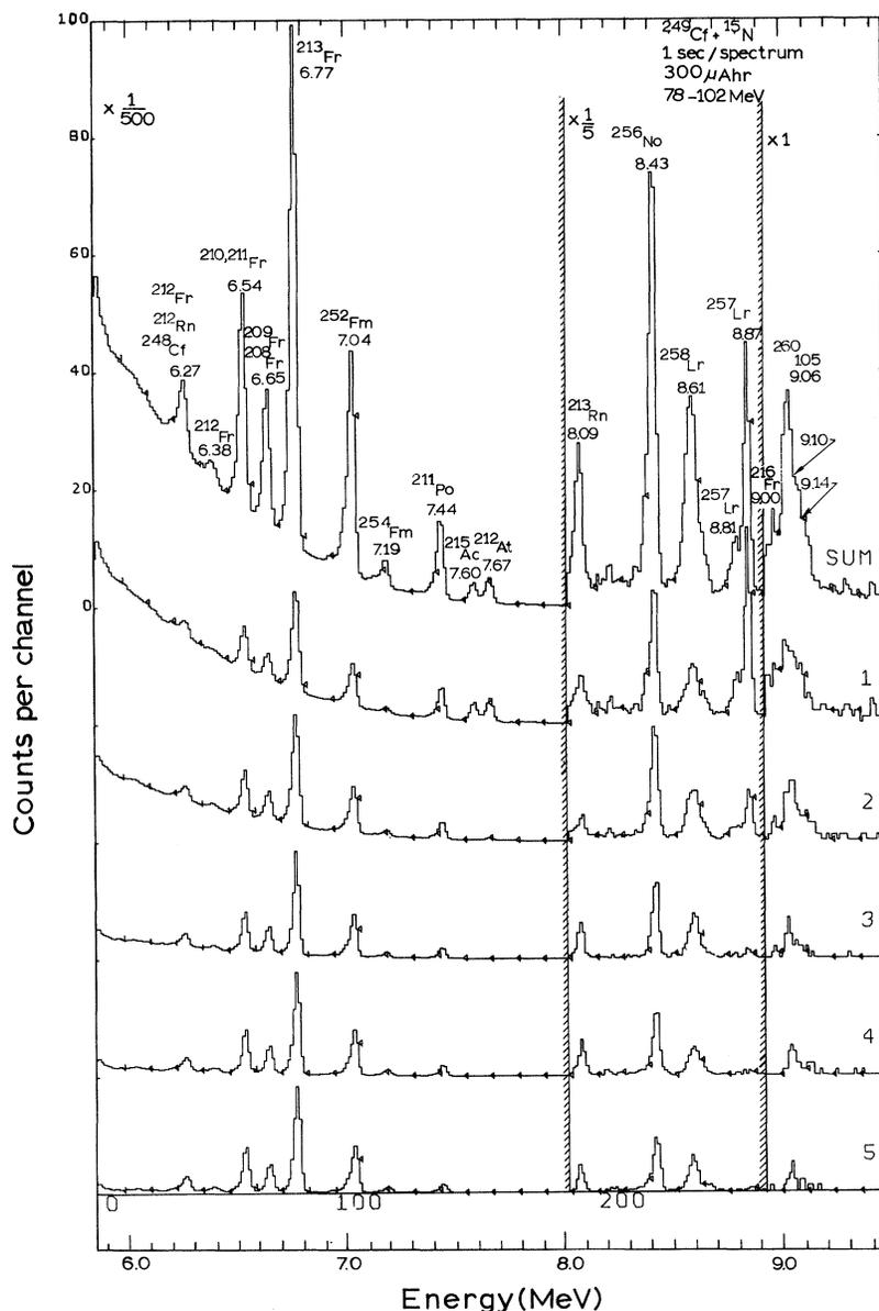
FIG. 1. A series of alpha-particle spectra produced by bombardments of  $^{249}\text{Cf}$  with  $^{15}\text{N}$  ions. The alpha peak at 9.00 MeV is that of  $^{216}\text{Fr}$ , the daughter of 23-msec  $^{220}\text{Ac}$  produced from the lead impurity in the target. Most of the  $^{211}\text{Po}$  derives from electron-capture of 7.2-h  $^{211}\text{At}$ .
