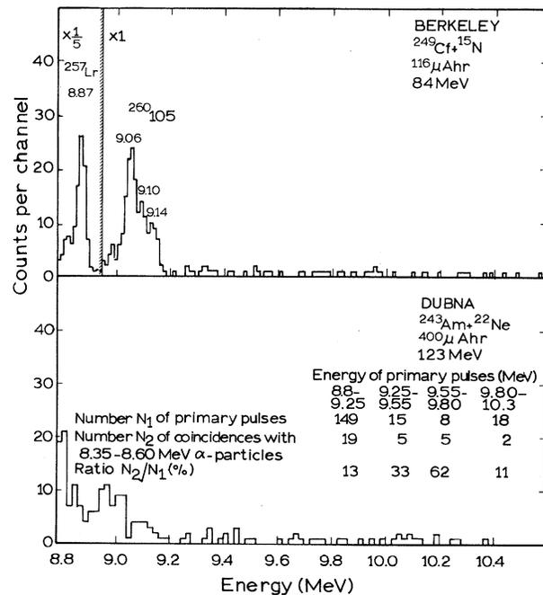
FIG. 4. A comparison of the alpha-particle spectra produced in the Dubna experiments (Refs. 11 and 12) with those reported in this paper.
