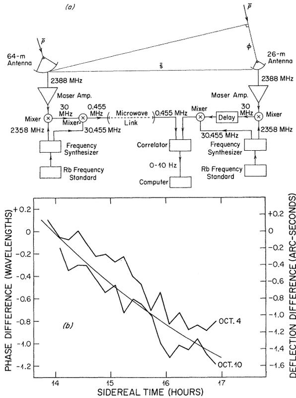
FIG. 1. (a) Schematic block diagram of the interferometer system. (b) Observations of the relative phase difference between the two radio sources on 4 and 10 October 1969. The smooth curve shows the baseline from the solution for  $a$ ,  $b$ , and  $c$  obtained from all of the data.
