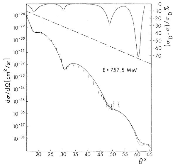
FIG. 1. Cross section for elastic scattering of 750-MeV electrons on Ca<sup>40</sup> as a function of scattering angle  $\theta$  calculated from the shell-model charge distribution of Ref. 4 with (dashed line) and without (solid line) dispersion effects. The upper part of the figure shows the relative effect of the dispersion terms,  $(\sigma_D - \sigma) / \sigma_D$ . The experimental data are from Ref. 3.
