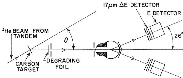
FIG. 1. A schematic representation of the double-scattering system.
