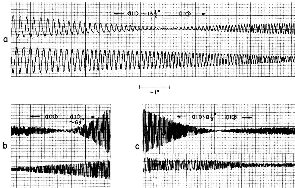
FIG. 2. Rotation diagrams in the  $\langle 110 \rangle$  plane at 50.85 kG and  $\sim 1$  K for pure Cu (upper traces) and Cu + 34 ppm Cr (lower traces). (a) Neck oscillations,  $\sim 63^\circ$  to  $73^\circ$ ; (b) belly,  $\sim 46.5^\circ$  to  $50^\circ$ ; (c) belly,  $\sim 61^\circ$  to  $66.5^\circ$ ; all angles measured from  $\langle 100 \rangle$ . The small horizontal steps in the oscillations derive from the windings on the potentiometer used to indicate angle, and hence are spurious.
