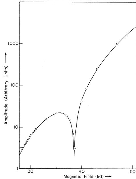
FIG. 1. Experimentally determined amplitudes for the  $\langle 111 \rangle$  belly in Cu+34 ppm Cr at ~1 K, and fitted curves of the form  $A(H, T, x) | \cos(\pi \Delta F/H) |$  (solid and dashed) and  $A'(H, T, x) | \cos[(\pi/2)(g m^*/m_0 - 2\Delta F'/H)]$  (solid line).
