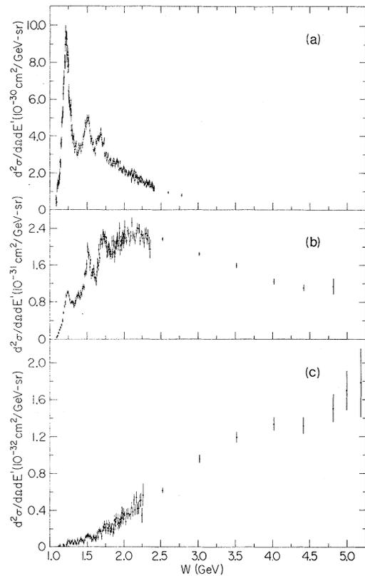
FIG. 2. Three representative radiatively corrected spectra at (a)  $\theta = 6^\circ$ ,  $E = 7$  GeV; (b)  $\theta = 6^\circ$ ,  $E = 16$  GeV, and (c)  $\theta = 10^\circ$ ,  $E = 17.7$  GeV. The ranges of  $q^2$  covered are (a)  $0.2 \leq q^2 \leq 0.5$  ( $\text{GeV}/c$ ) $^2$ ; (b)  $0.7 \leq q^2 \leq 2.6$  ( $\text{GeV}/c$ ) $^2$ ; and (c)  $1.6 \leq q^2 \leq 7.3$  ( $\text{GeV}/c$ ) $^2$ . The elastic peaks are not shown.
