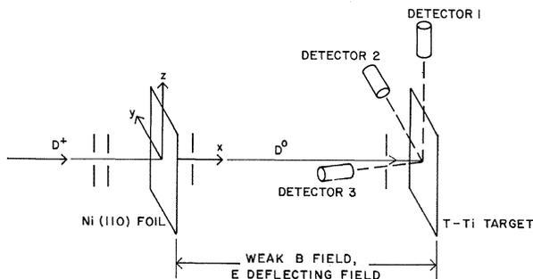
FIG. 1. Schematic diagram of experimental arrangement.
