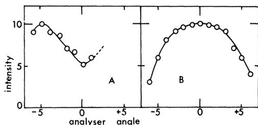
FIG. 3. The emission current plotted as a function of rotation of the analyzer. The scales are proportional to intensity and angle but have not been calibrated. (a) Copper  $\langle 111 \rangle$ ; (b) tungsten  $\langle 110 \rangle$ .
