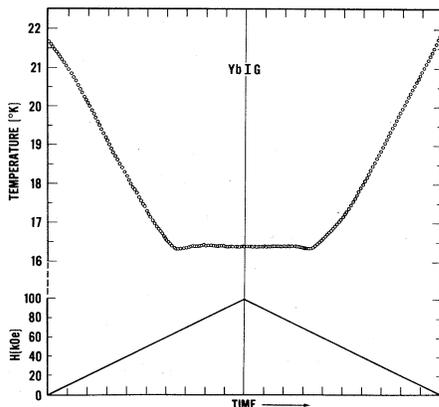
FIG. 1. The change in temperature of ytterbium iron garnet with field. As the field is increased the temperature falls from near 22°K to 16.5°K. A decrease in the field returns the temperature to its initial value. No temperature change is observed above  $H_l = 65$  kOe. Above this field the system is in the angled phase.
