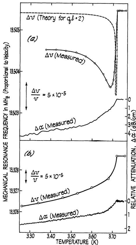
FIG. 1. Relative velocity and attenuation measurements as a function of temperature for 13-MHz sound along [001] in tin. (a) Data for shear waves with polarization along [110], also showing the theoretical curve of Ozaki and Mikoshiba for  $ql=2$ . (b) Compressional-wave data. Note that  $\Delta v/v = (v_n - v_s)/v_n$ .
