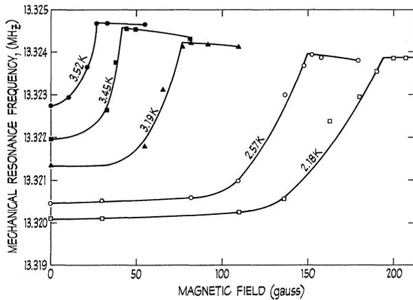
FIG. 2. Magnetic field variation of the mechanical resonance frequency (which is proportional to the sound velocity) of 13.3-MHz compressional waves propagating along [001] in tin for several temperatures below  $T_c$ .
