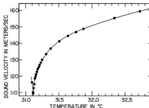
FIG. 1. The velocity of sound in  $\text{CO}_2$  at a density of  $0.467 \pm 0.001 \text{ g/cm}^3$  as a function of temperature in the one-phase region.
