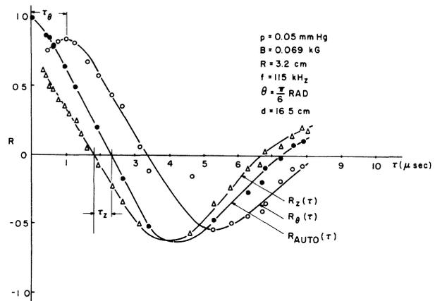
FIG. 1. Experimentally determined auto- and cross-correlation functions.
