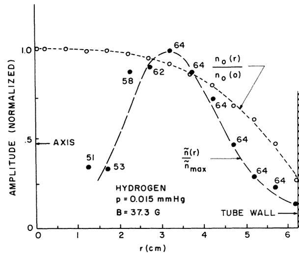
FIG. 3. Measured radial dependence of the fluctuating and steady-state components of the ion density  $\tilde{n}$  and  $n_0$ , respectively (normalized to their maximum values).
