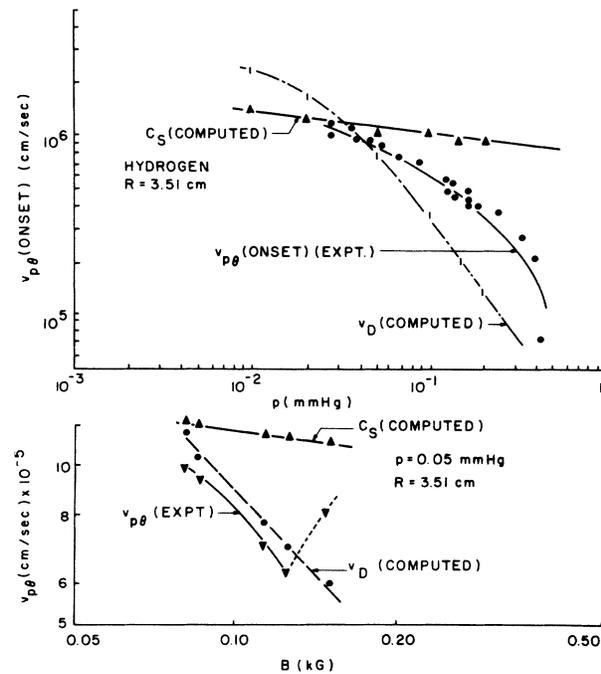
FIG. 2. Parametric dependence of  $v_{p\theta}$ ,  $v_D$ , and  $c_s$  on the magnetic field  $B$  and neutral-gas pressure  $p$ .
