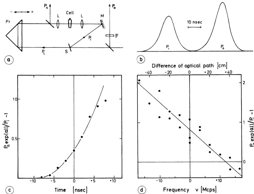
FIG. 1. (a) Schematic of the experimental system. (b) Oscilloscope trace depicting the incoming signal  $P_i$  and the amplified signal  $P_a$ . (c) Amplification versus time (at  $\nu = \omega/2\pi = 0$ ) for a solution of iodine in  $\text{CCl}_4$  ( $\alpha = 0.07 \text{ cm}^{-1}$ ). (d) Amplification at the pulse maximum versus frequency difference.
