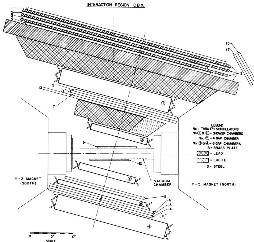
FIG. 1. Schematic of the spark-chamber detector.
