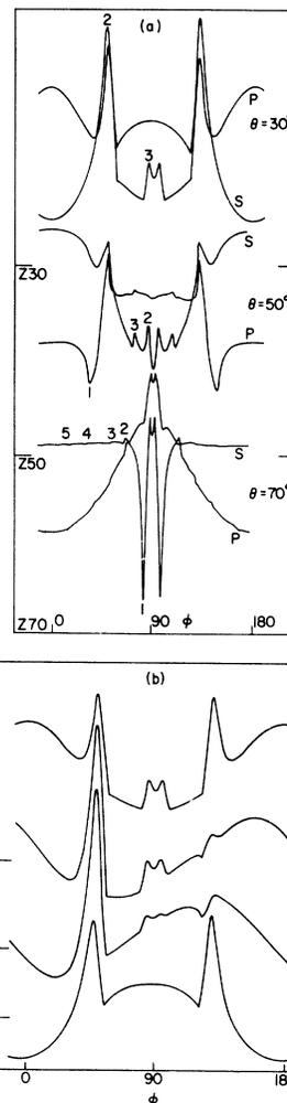
FIG. 2. (a) Typical rotation curves of reflected intensity versus  $\varphi$  for  $s$  and  $p$  polarized light.  $\lambda = 0.526 \mu$  and  $\theta = 30^\circ, 50^\circ, 70^\circ$ . (b) Rotation of the incident polarization from  $s$  to  $p$  in  $30^\circ$  steps.  $\lambda = 0.526 \mu$ .
