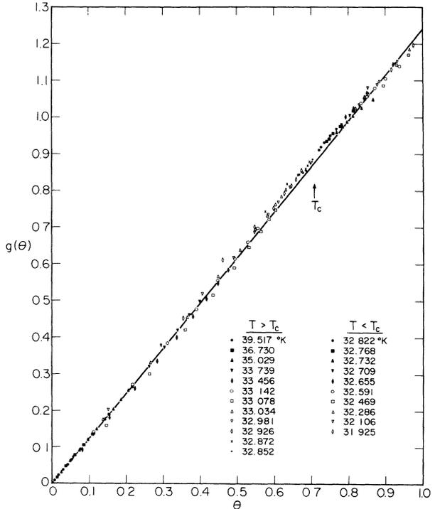
FIG. 2. A plot of the function  $g(\theta)$  in the parametric equation of state, Eq. (5), obtained from an analysis of our  $\text{CrBr}_3$  data with  $a = 1.1$ . The line has the equation  $g(\theta) = 1.24\theta$ .
