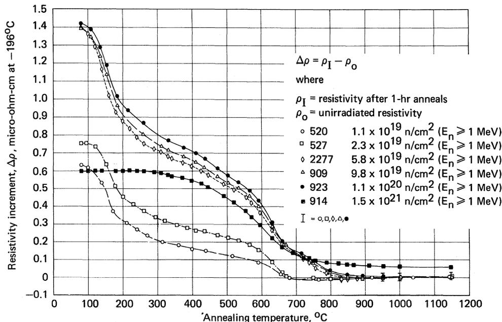
FIG. 2. Isochronal resistivity recovery of neutron-irradiated, recrystallized molybdenum as a function of annealing temperature.
