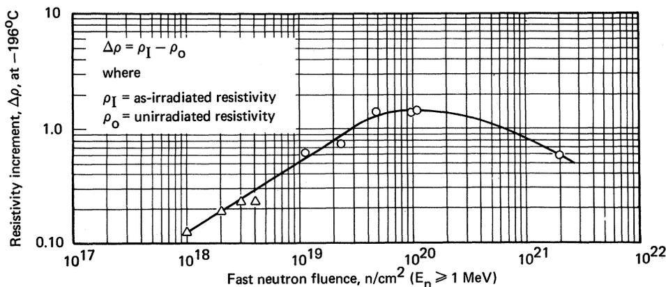
FIG. 1. Total radiation-induced resistivity increment for molybdenum as a function of fast-neutron fluence (dotted circles, data taken in this study; dotted triangles, Ref. 1).
