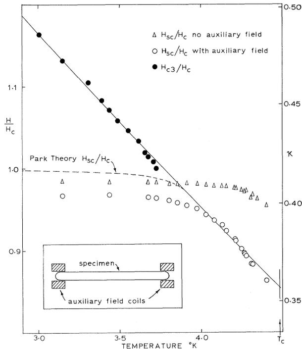
FIG. 1. Effect of auxiliary-field coils placed at the ends of the specimen (see inset) on the observed supercooling field  $H_{SC}$ . The specimen is an electropolished single-crystal cylinder of tantalum. The full line is a curve of  $H_{C3}/H_C$  obtained from the measurements, as described in the text. The  $\kappa$  scale applies only to this curve.
