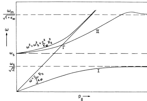
FIG. 1. Schematic dispersion relation for surface-plasmon oscillations in an idealized metal-semiconductor junction (see text).  $\Gamma$  corresponds to a frequency  $\sim(\omega_M\omega_S)^{1/2}$ .
