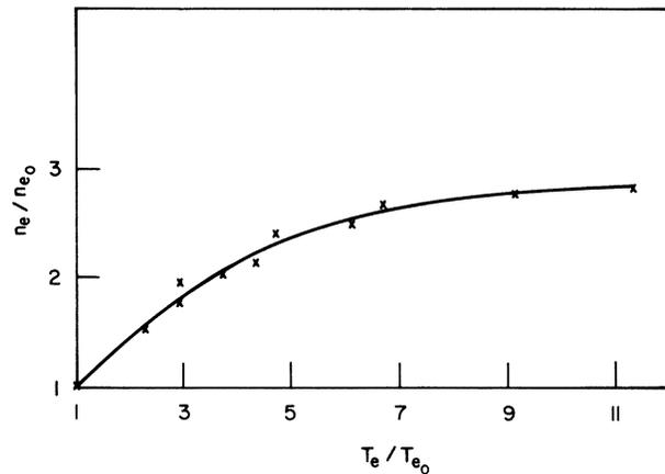
FIG. 2. Typical plot of electron density at 150  $\mu\text{sec}$  of microwave heating versus electron temperature during heating. Each has been normalized to the respective unperturbed value for this particular afterglow time. ( $T_{e0} \sim 170^\circ\text{K}$  for this plot, gas temperature of 77°K and pressure of 9.5 Torr.)
