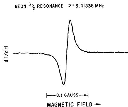
FIG. 1. Derivative of transmitted light intensity at 640.2 nm, with respect to magnetic field, versus field intensity. The lock-in time constant is 1 sec. Cell contains 0.01 Torr neon and 0.2 Torr helium.
