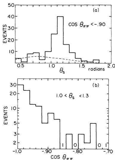
FIG. 2. Data obtained from a 4-in.-thick tungsten regenerator placed at five different positions in the decay volume. (a) Distribution of the smaller of the opening angles of the two pairs of  $\gamma$  rays for events with collinearity  $\cos\theta_{\pi\pi} < -0.90$ . The dashed line is the background estimated from the free-decay distribution. (b) Collinearity distribution for those events with the smaller opening angle between 1.0 and 1.3 rad.
