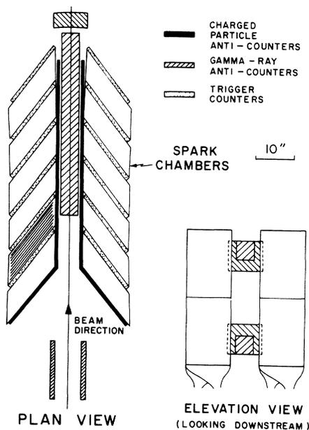
FIG. 1. Plan view of the experimental apparatus. An elevation view of the counter arrangement is shown in the insert.
