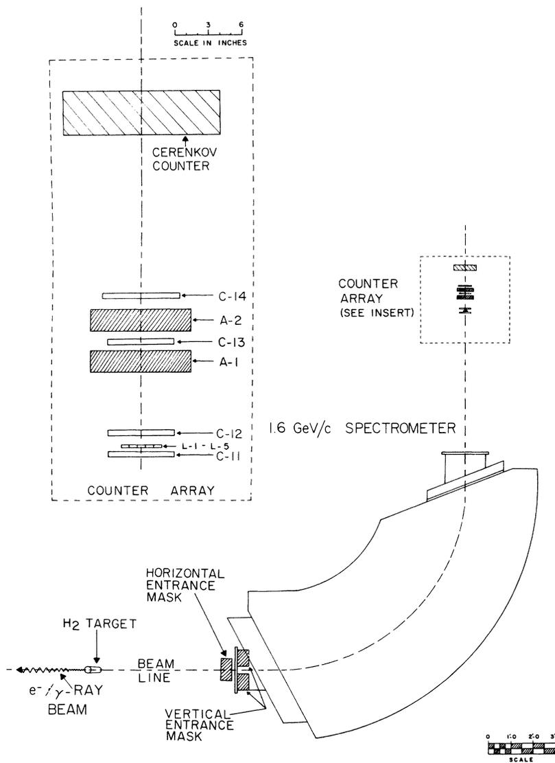
FIG. 1. Positioning of the spectrometer and counters relative to the beam line and target. The insert shows an enlarged picture of the counter array.
