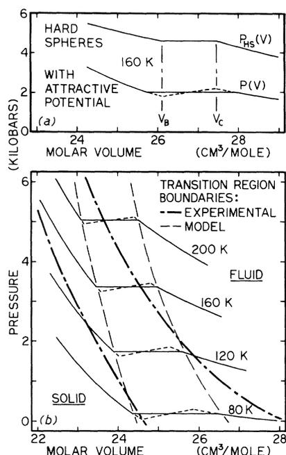
Fig. 2. (a) Hard-sphere isotherm through the solid-fluid transition and the corresponding isotherm obtained when an attractive potential is included (see text). (b) Solid-fluid phase transition calculated from the model, compared with the experimentally determined transition region.
