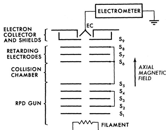
FIG. 1. Schematic diagram of the electron gun.
