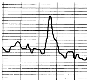
FIG. 1. Recording of the N=1 \rightarrow 3, \Delta J=0 rotational line of O_2 at 424 763.80. The linewidth is approximately 4 Mc/sec.
