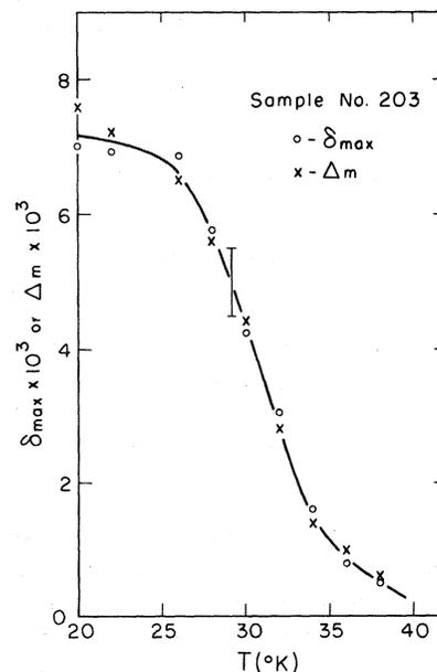
FIG. 2. Effect of 10-min isochronal anneals at indicated temperatures on data of Fig. 1.  $\Delta_m$  is  $2[f - f(\text{background})]/2063$ .
