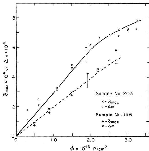
FIG. 3. Growth of an anelastic process near 10°K with integrated proton flux. Sample 203 is a single crystal with stress parallel to  $\langle 111 \rangle$  axis; sample 156 is a polycrystalline wire.
