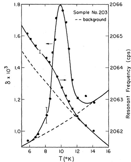
FIG. 1. Temperature dependence of internal friction  $\delta$  and fundamental frequency of a cantilevered Cu single crystal. Longitudinal stress is parallel to  $\langle 111 \rangle$  crystallographic axis. Background frequency curve based on post-anneal results.
