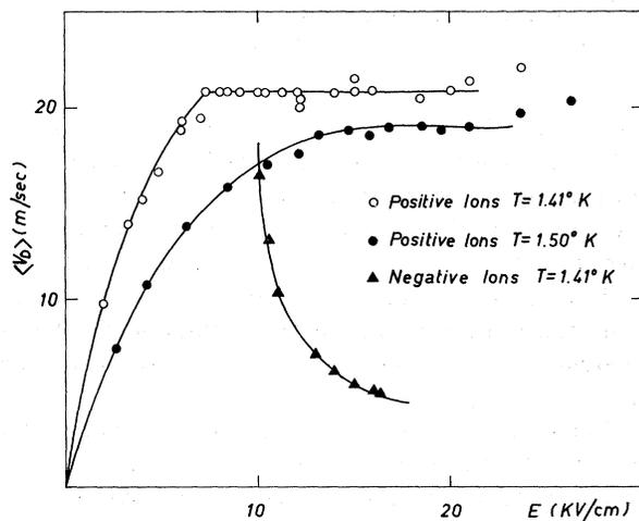
FIG. 1. Drift velocity  $\langle V_D \rangle$  of ions as a function of electric field at high temperatures. As we can see, the positive and negative ions behave in a different manner.
