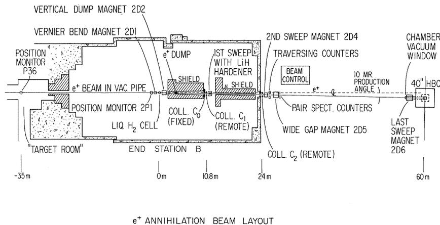
FIG. 1. Layout of the positron annihilation beam used in the experiment.
