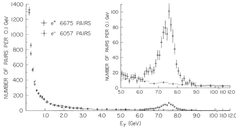
FIG. 2. Measured pair spectrum for  $e^+$ - and  $e^-$ -induced radiation. The  $e^+$ -induced spectrum is that actually measured while the  $e^-$  has been normalized to have a bremsstrahlung component equal to that of the  $e^+$  spectrum in the energy interval 0.4-5.0 GeV. The inset shows the annihilation enhancement at  $\sim 7.5$  GeV.
