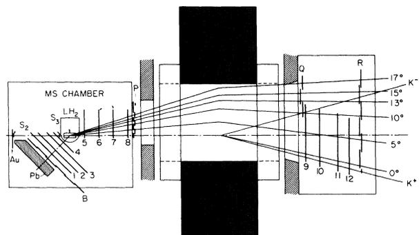
FIG. 1. The experimental apparatus drawn to scale.  $MS_{1-4}$ ,  $MS_{5-8}$  and  $MS_{9-12}$  are digitized wire spark chambers. Arrays  $B$ ,  $P$ , and  $R$  are the triggering counters. Typical trajectories through the system are shown.
