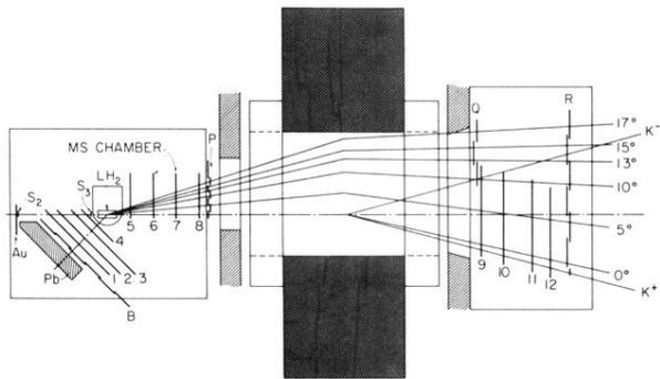
FIG. 1. The experimental apparatus drawn to scale.  $MS_{1-4}$ ,  $MS_{5-8}$  and  $MS_{9-12}$  are digitized wire spark chambers. Arrays  $B$ ,  $P$ , and  $R$  are the triggering counters. Typical trajectories through the system are shown.
