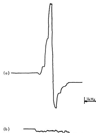
FIG. 3. Typical 6.835-GHz light-modulation signals for 7800-Å  $D_2$  Rb<sup>85</sup> light; (a) with a circular analyzer; (b) without a circular analyzer. The vertical scale is the output of the 30-MHz balanced mixer in arbitrary units. The detection-system bandwidth was 1 Hz.
