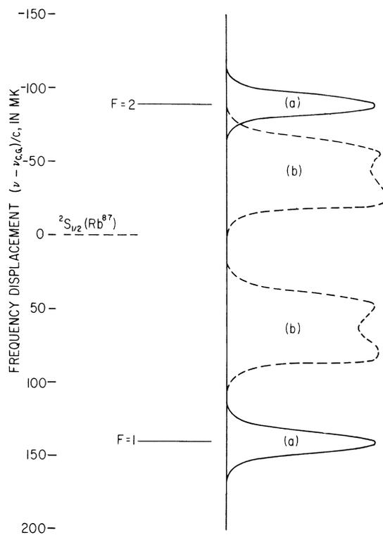
FIG. 1. (a) The optical absorption lines of Rb<sup>87</sup> and (b) a typical spectral profile of a Rb<sup>85</sup> lamp. More detailed experimental studies of spectral profiles in the rubidium isotopes can be found in H. M. Gibbs and R. J. Hull, Phys. Rev. **153**, 132 (1967).
