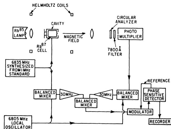
FIG. 2. The experimental apparatus.
