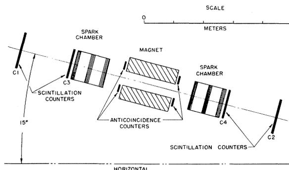
FIG. 1. Schematic elevation view of the spectrograph.
