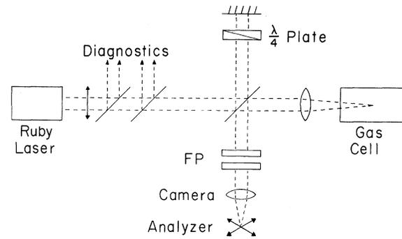
FIG. 1. Experimental arrangement for observation of stimulated thermal Rayleigh scattering in gases.
