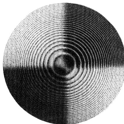
FIG. 2. Interferogram of stimulated thermal Rayleigh-scattered light from a  $\text{CO}_2 + \text{NO}_2$  gaseous mixture at the density of 71 amagat. Measured  $\alpha = 0.025 \text{ cm}^{-1}$  at  $\lambda = 6943 \text{ \AA}$ , and interferometer spacer of 100 mm was used. The lighter sectors are due to STRS light and the darker sectors the incident laser light.
