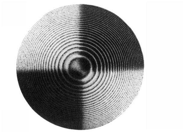
FIG. 2. Interferogram of stimulated thermal Rayleigh-scattered light from a  $\text{CO}_2 + \text{NO}_2$  gaseous mixture at the density of 71 amagat. Measured  $\alpha = 0.025 \text{ cm}^{-1}$  at  $\lambda = 6943 \text{ \AA}$ , and interferometer spacer of 100 mm was used. The lighter sectors are due to STRS light and the darker sectors the incident laser light.
