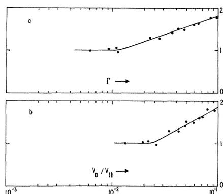
FIG. 1. The ratio of Thomson-scattering temperature to conductivity temperature plotted against (a) the runaway parameter  $\Gamma$ , and (b) the ratio of electron drift to thermal velocity.
