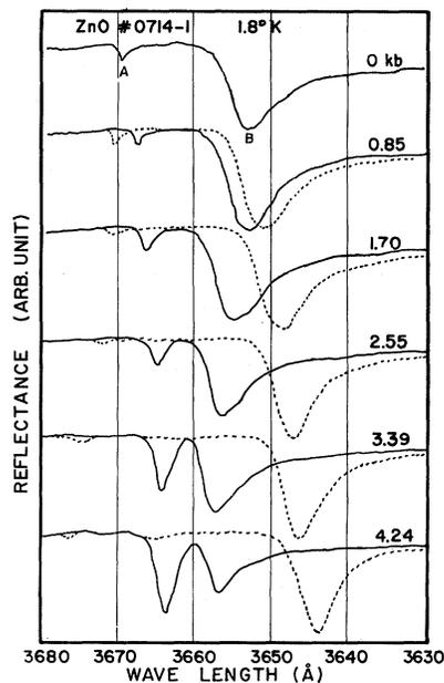
FIG. 1. The change of the reflection spectra of ZnO for  $\vec{P} \perp C$  and  $\vec{k} \parallel C$ . Solid and broken lines indicate the components polarized with  $\vec{E} \parallel \vec{P}$  and  $\vec{E} \perp \vec{P}$ , respectively
