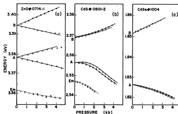
FIG. 2. Splitting of the  $A$  and  $B$  exciton lines in ZnO, CdS, and CdSe. Open and closed circles represent the experimental positions of the split components polarized with  $\vec{E} \parallel \vec{P}$  and  $\vec{E} \perp \vec{P}$ , respectively. Shifts of emission lines in ZnO and CdS are shown by the broken lines. (Definition of the  $A$  and  $B$  lines in ZnO indicated follows Thomas, Ref. 2.)
