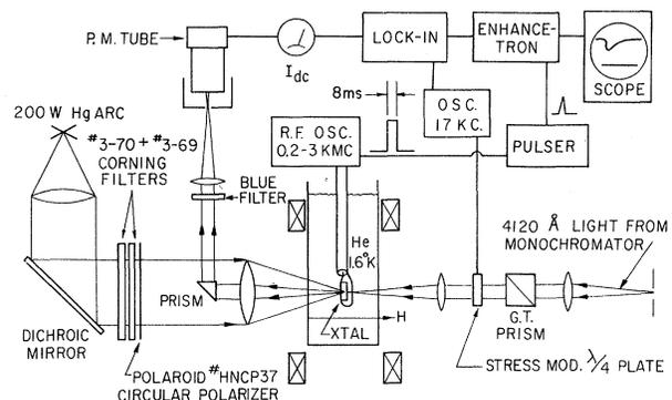
FIG. 2. Experimental arrangement for ENPOPS, showing optical system for measuring  $P_e$  and  $P_n$ .
