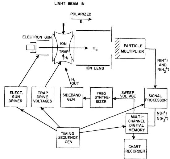
FIG. 2. Experimental block diagram.
