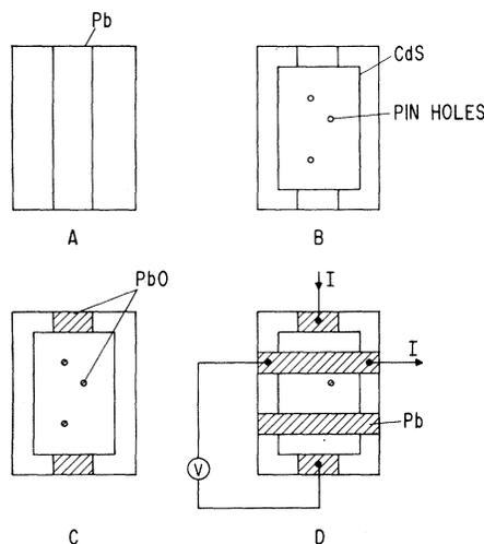
FIG. 1. Sample preparation. (a) An evaporated Pb film on a glass slide. (b) A CdS film has been deposited on top of the Pb film. Normally the CdS film will not be continuous but contain small pinholes. (c) The sample is oxidized such that an insulating layer of PbO can be formed in the pinholes. (d) Cross strips of Pb have been evaporated to complete the tunnel junctions.
