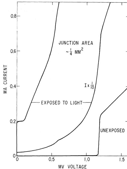
FIG. 3. A typical Sn-CdS-Sn sample characteristic at 2.2°K. The CdS layer is approximately 75 Å thick. The dc Josephson current is clearly visible after the junction has been exposed to light. Note current onset at approximately half the energy gap in the exposed curve.
