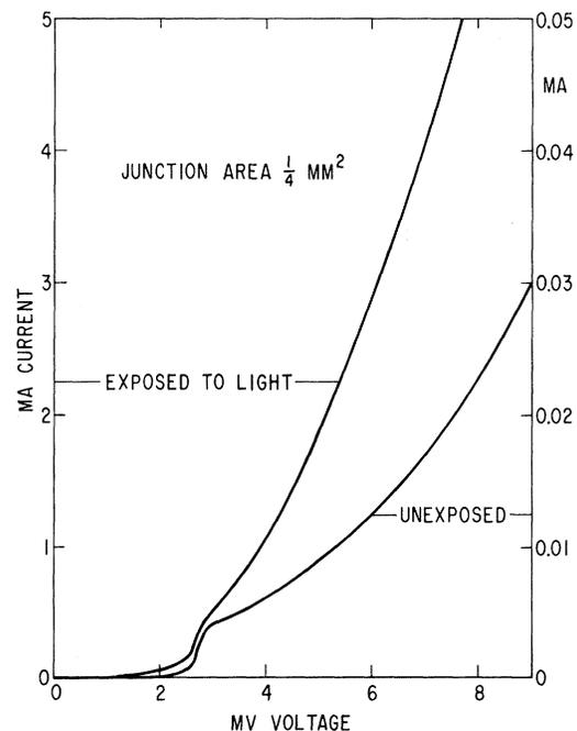
FIG. 2. A typical Pb-CdS-Pb sample characteristic at 2.2°K. The CdS layer is approximately 200 Å thick. Note the current onset at approximately half the energy gap in the exposed curve.
