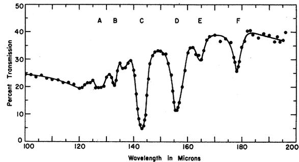
FIG. 1. Transmission spectrum of boron-doped germanium at  $\sim 5^\circ\text{K}$ . Room temperature resistivity = 14 ohm cm. Sample thickness = 3.5 mm.
