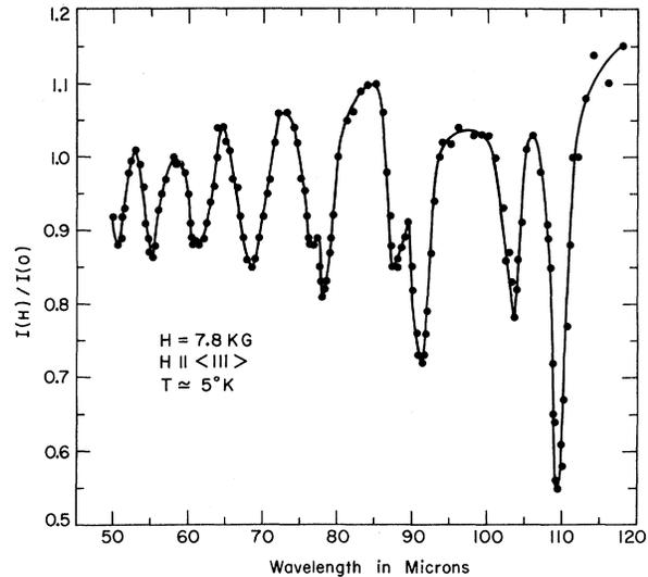
FIG. 3. Effect of a magnetic field on the ionization absorption of boron in germanium. The ordinate is the ratio of transmitted intensity through the sample with and without field.
