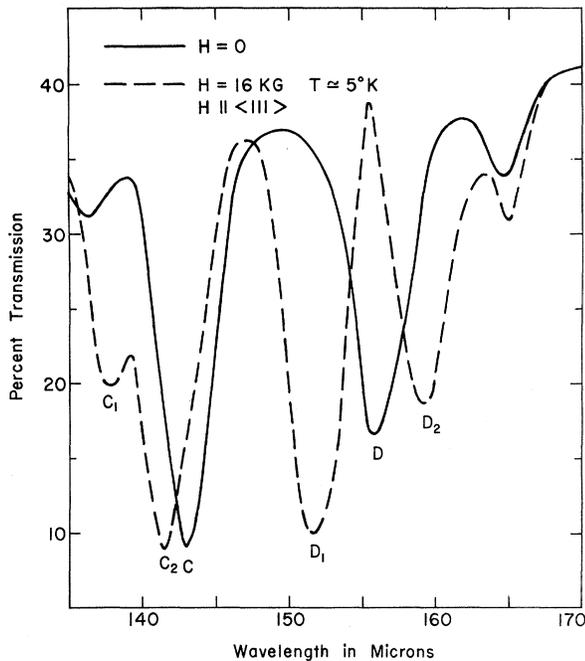
FIG. 2. Effect of a magnetic field on the two strong excitation lines of boron in germanium.
