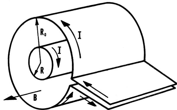
FIG. 1. Basic cylindrical punch configuration showing the magnetic field and the currents in coil and plasma.
