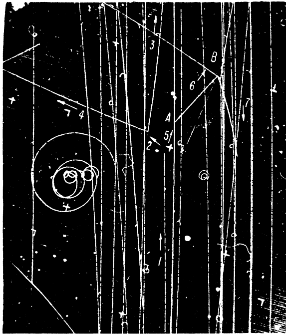
FIG. 3. The primary reaction is \pi^- (Track 1) + p \rightarrow \Lambda (arrow No. 5) + K^0 (arrow No. 2). The K^0 decays into a \pi^- (Track 3) and a \pi^+ (Track 4). The \Lambda subsequently interacts at point A to produce a \Sigma^+ (Track 6) plus a neutron. The \Sigma^+ decays at point B into a \pi^+ (Track 7) and a neutron.
