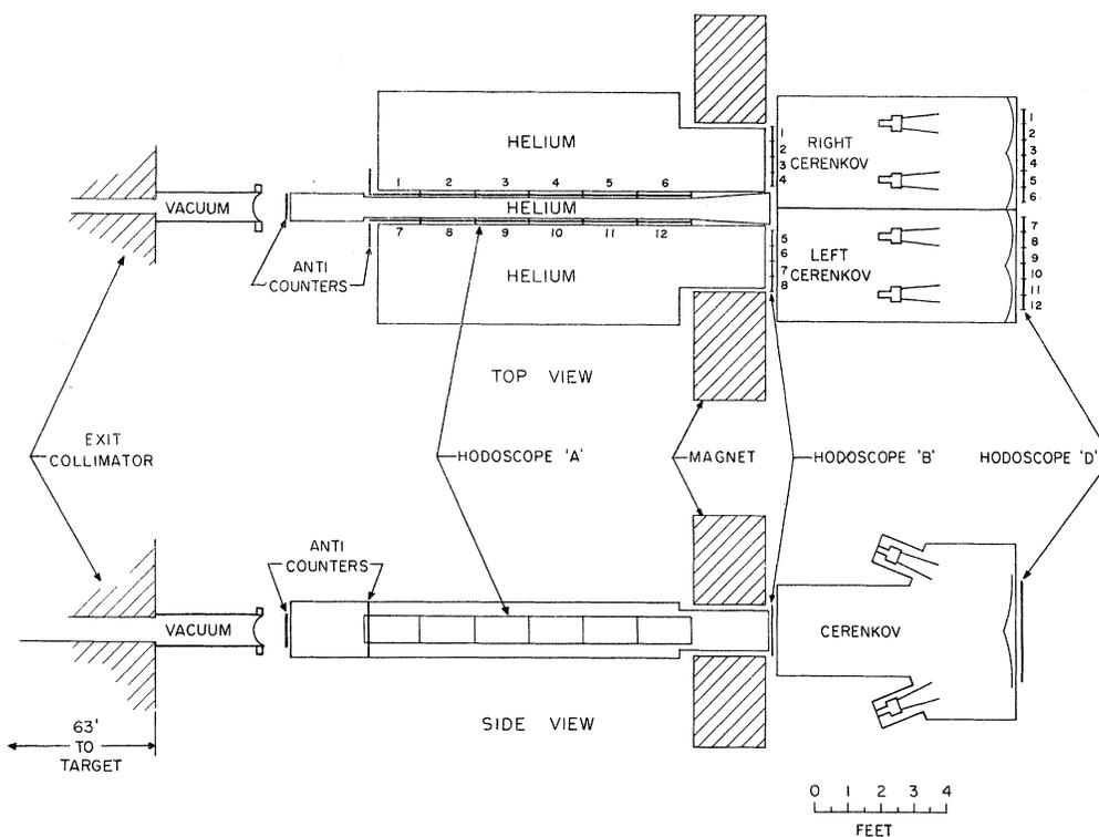
FIG. 1. Vertical and horizontal views of the detection apparatus.
