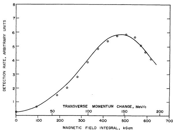
FIG. 2. Event rate as a function of the magnetic field in the analyzing magnet. The abscissa is labeled by the transverse momentum change produced by this field. The Monte Carlo predictions for  $K_{e3}$  (full curve) are shown as well as the experimental results (points with error flags).
