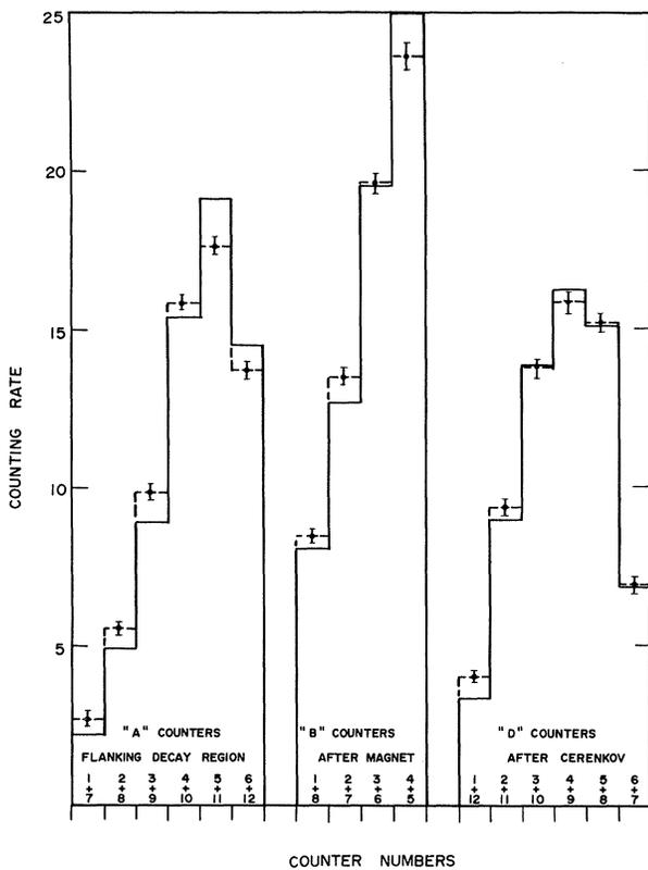
FIG. 3. Distribution of events in the hodoscope counters. The rates in symmetrically placed counters are combined. The experimental results (full line) are compared with the Monte Carlo predictions (dashed).
