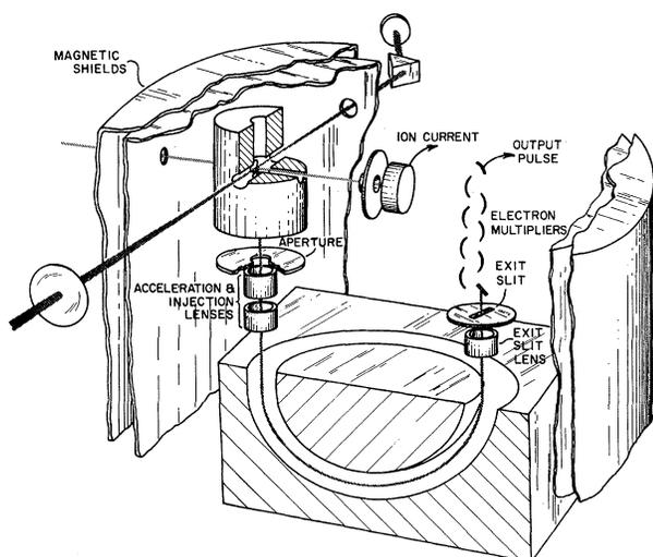
FIG. 2. Detail of the interaction chamber and electron analyzer. To increase the useful solid angle, and to minimize the effect of patch fields, the electrons are accelerated to 11.2 eV for analysis. The nominal trajectory has about 5.7 cm radius. All critical surfaces are copper.
