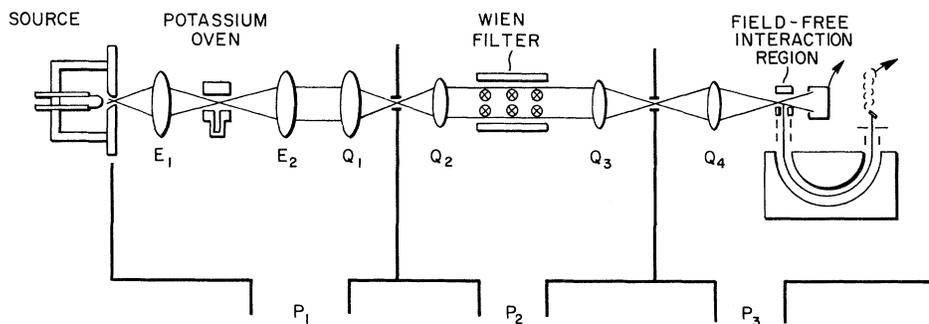
FIG. 1. Block diagram of the ion-beam apparatus.  $E_1$  and  $E_2$  are "Einzel" lenses. The symbol  $Q$  represents a 12-element symmetrical quadrupole lens. The operating pressure in the interaction chamber is held to  $10^{-8}$  Torr or less by the 200-liter/sec ion pump,  $P_3$ .
