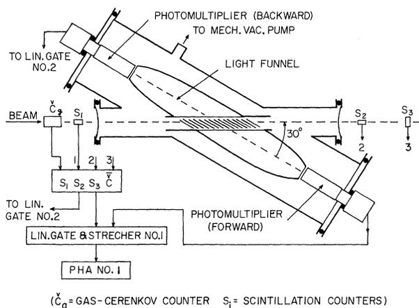
FIG. 1. Sketch of the experimental setup and block diagram of the electronics.
