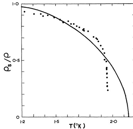
FIG. 1. Values of  $\rho_s/\rho$  for the present Vycor specimen, normalized to the value 0.93 at  $1.2^\circ\text{K}$ . The solid curve gives Andronikashvili's values of  $\rho_s/\rho$  for the bulk liquid.
