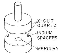
FIG. 1. The construction of a metal sample for hypersonic-attenuation measurements.
