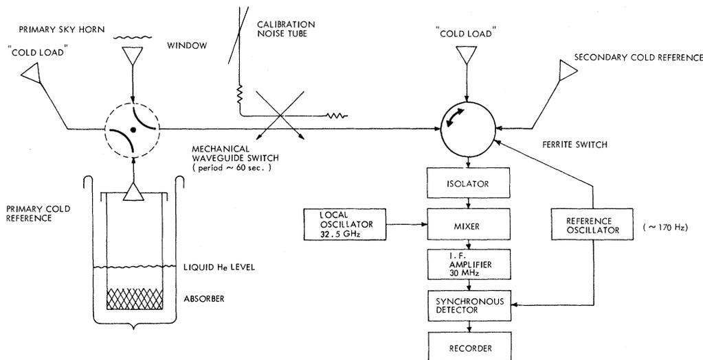
FIG. 1. Radiometer block diagram for absolute measurements.
