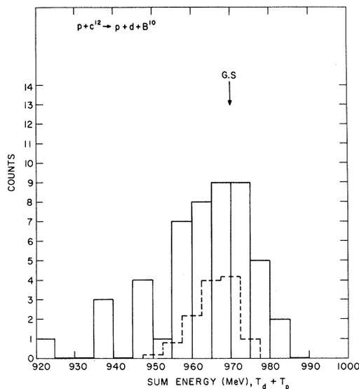
FIG. 3. Sum-energy spectrum,  $T_p + T_d$ , for all coincident events in which the ratio of proton to deuteron kinetic energies,  $T_p/T_d$ , lies between 0.084 and 0.145. The dashed curve is the sum-energy resolution as determined from free  $p$ - $d$  coincidences. This curve has been displaced by 27 MeV, which is the binding energy of the deuteron in the  $^{12}\text{C}$  nucleus. The arrow G. S. shows the location of the ground state of  $\text{B}^{10}$ .
