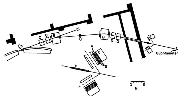
FIG. 1. Schematic drawing of the transport system and the detection apparatus.  $H$ , hydrogen target;  $T$ , thin-foil optical spark chambers;  $S$ , scintillation counters;  $C$ , Cherenkov counters.
