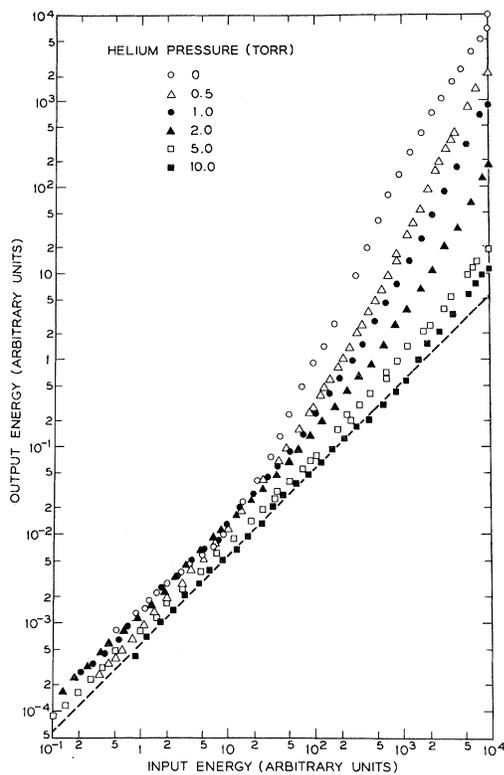
FIG. 3.  $E_0$ , as a function of  $E_i$ , for 0.02 Torr  $\text{SF}_6$  showing the effect of helium buffer gas at various pressures. Notice the increase in  $P_{\text{th}}$  as helium pressure increased. (The maximum output point corresponds to no  $\text{SF}_6$  in the absorption cell.)
