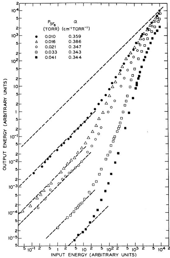
FIG. 1.  $E_0$ , as a function of  $E_i$ , for transmission through 9.4 m length of various  $\text{SF}_6$  pressures. The maximum  $E_i$  and  $E_0$  (without  $\text{SF}_6$ ),  $10^4$  on the arbitrary scale, corresponds to a peak input intensity of  $\sim 10^4 \text{ W cm}^{-2}$ . The absorption coefficients,  $\alpha$ , are obtained from the linear portions of the curves at the low end of the input energy scale. (The maximum  $E_0$  corresponds to no  $\text{SF}_6$  in the absorption cell.)
